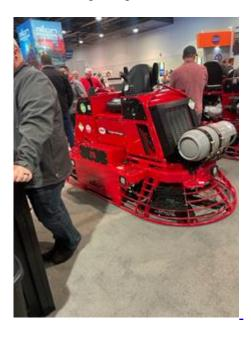
Allen Engineering's new riding concrete trowel, model HDX615, powered by Power Solutions International's 2.4-liter dual-fuel gasoline and propane engine, was unveiled during World of Concrete 2023.
